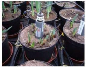
A Delta-T theta probe measuring soil moisture
